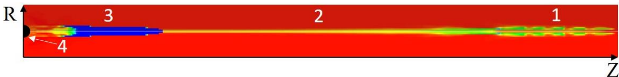
Figure 1. Spatial structure of waves in the M_A=0.2 mode: 1 - Alfvén wave; 2 - extended "tail" of Alfvén wave; 3 - slow magnetosonic wave; 4 – source that generates a sequence of laser plasma bunches.
