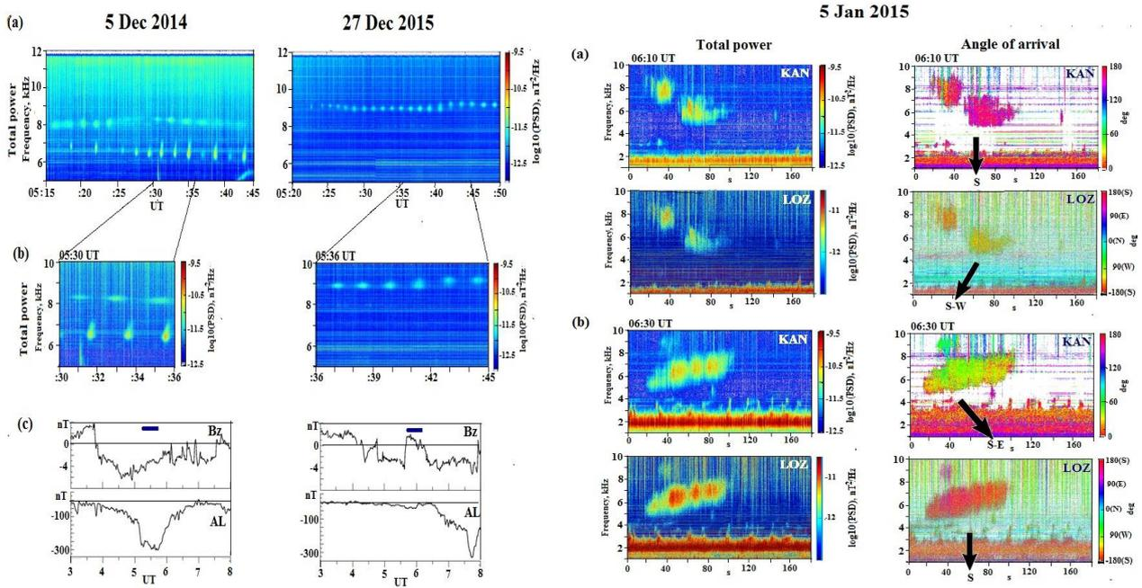
**Figure 3.** Left part – two VLF events with QP repetition and IMF Bz and AL-index variation during these events. The right part - two events of the “birds” at KAN and LOZ and the directions to their possible ionospheric exit areas.
