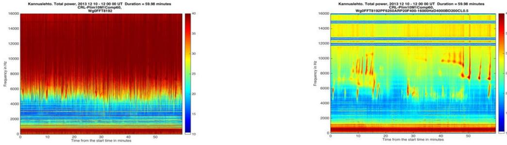
**Figure 1.** The example of 1-h spectrograms of VLF emissions at KAN: the non-filtered spectrogram (left panel) and the same spectrogram after sferics filtering (right panel). Three white high-frequency horizontal lines are the removed radio navigation transmitter signals.
