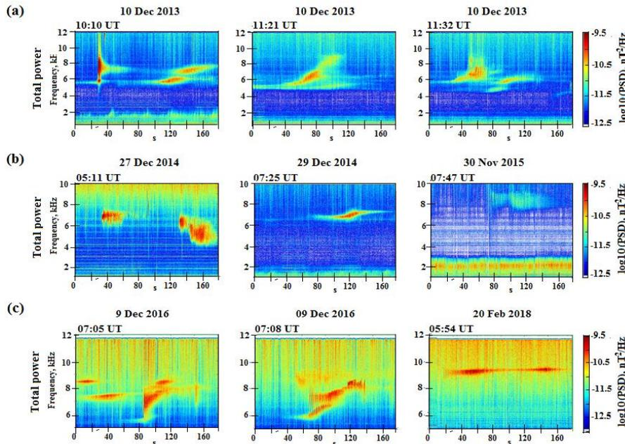
**Figure 2.** Examples of 3-min spectrograms of the VLF patches of different shapes at KAN: (a) VLF patches with sharp low frequency cutoff; (b) the most typical shape of VLF patches; (c) very complicated spectra of the VLF patches.
