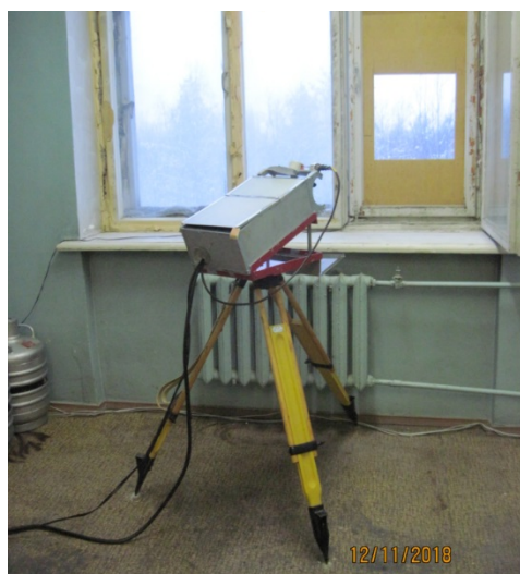
Figure 1. General view of a mobile microwave ozonemeter in Polar Geophysical Institute.
