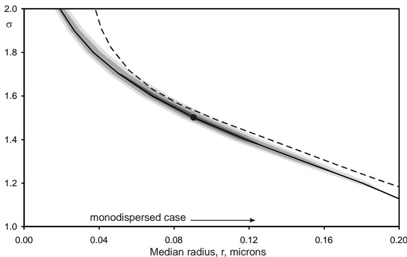
**Figure 5.** Retrieved characteristics of particle log-normal size distribution: solid line and gray areas (single, double and triple error) - twilight analysis (the same date as in Fig. 4), 21.4 km, dashed line - [Bourassa et al., 2008].
