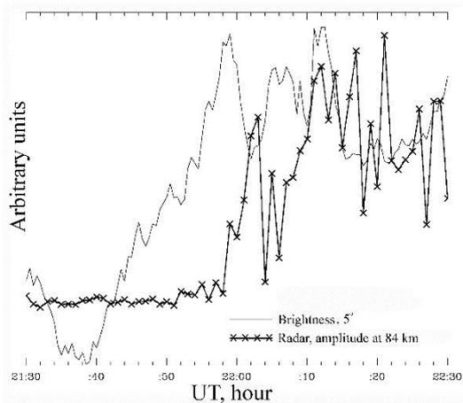
**Figure 3.** Sky luminescence variations in the circle with the radius of 5° above the radar (the simple line) and ordinary wave amplitude of the radar at the height of 84 km (the bold line with crosses).
