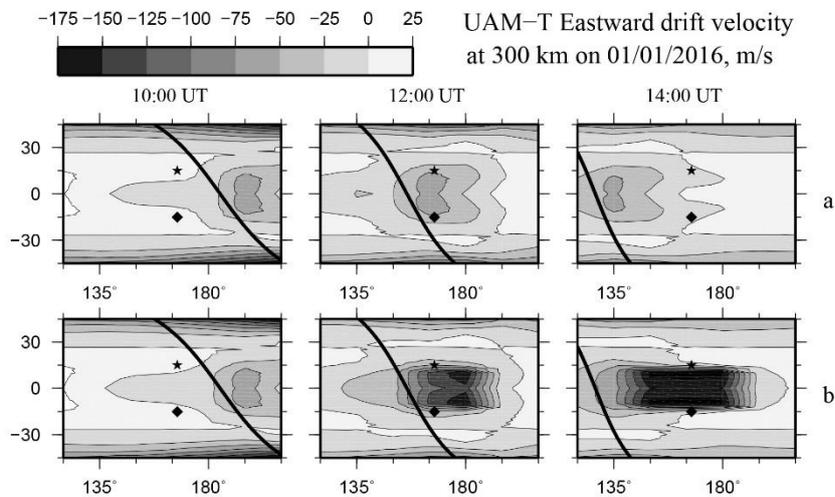
**Figure 2.** The UAM calculated eastward drift velocity (m/s) distributions at 300 km: **a)** without seismic currents; **b)**  $j_s = 20 \text{ nA/m}^2$ .
