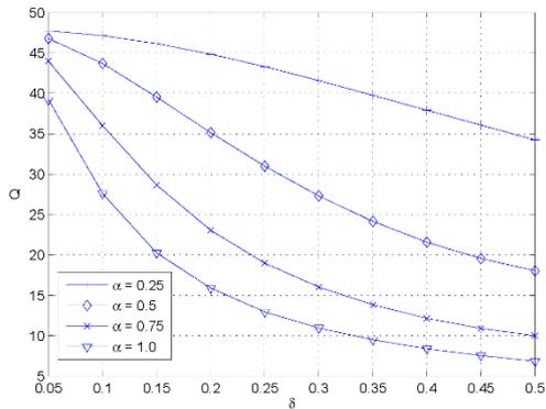
**Figure 3.** The dependence of the Q-factor of the resonator on  $\delta$  for  $A=1$ ,  $\Omega=1$ ,  $\gamma=0.01$ , and various  $\alpha$ .
