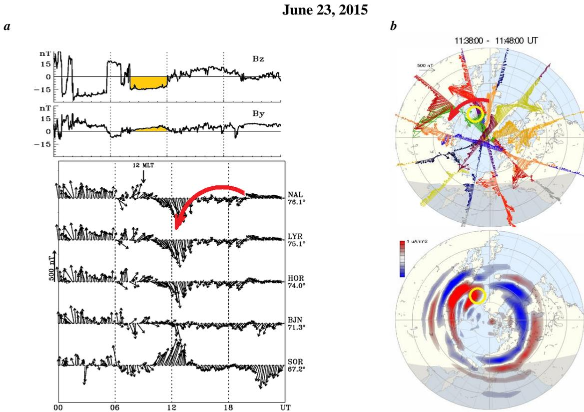
**Figure 3. a)** IMF  $B_z$  and  $B_y$  components and the horizontal vectors of the geomagnetic field; **b)** The AMPERE data: reduced magnetic field residual data showing the horizontal plane vector data of magnetic perturbation (*upper*); the radial current density (*bottom*). Upward currents are shown in red and downward currents in blue, yellow circle shows the position of the high latitude IMAGE stations.
