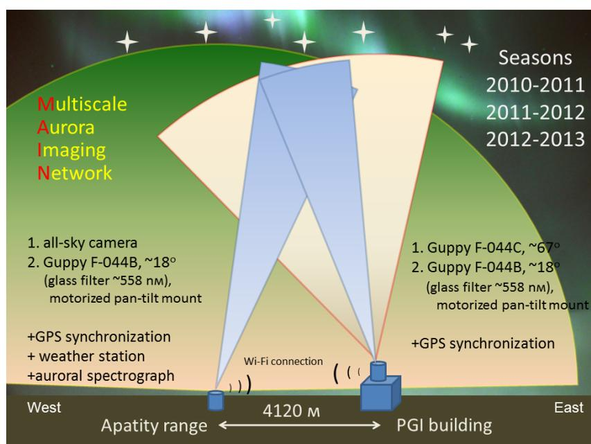
Fig. 1. Schema of the auroral camera network.
