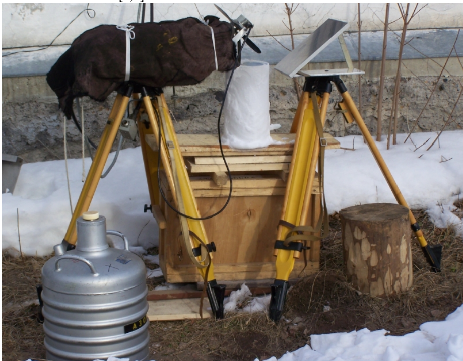
Fig. 1. The view of the microwave ozonemeter used in the measurements (twenty-four-hour observations) from March 14 till March 19, 2009.
