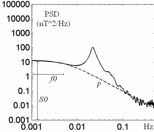
**Fig. 1.** An example of MEM power spectrum of  $B_y$  component (solid line) in the log-log scale and the approximation curve (dashed line) for June 14, 1999, 1200–1220 UT. The parameters of the approximation (1) are as follows:  $S_0=12.87 \text{ nT}^2/\text{Hz}$ ,  $f_0=0.005 \text{ Hz}$ ,  $P=1.7$ .
