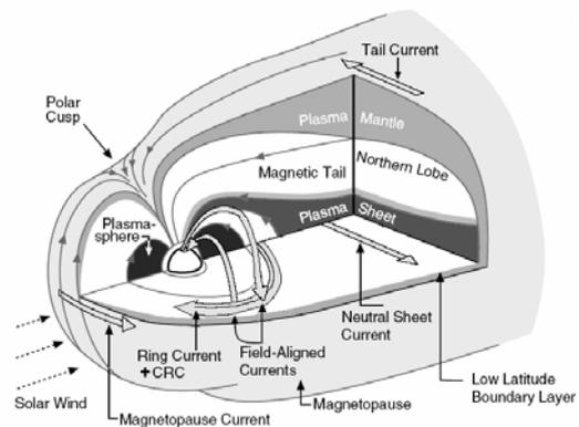
**Figure 6.** The improved structure of the main magnetospheric currents
