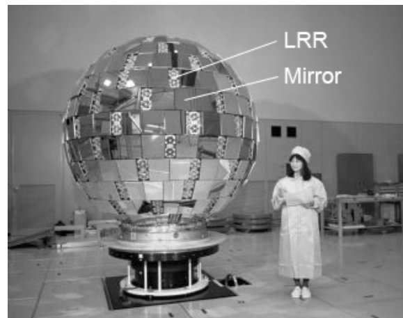
Fig. 1: Experimental geodetic satellite AJISAI.
