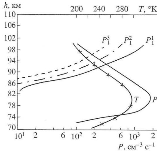
Fig. 1. Height distribution of temperature  $T$  for winter anomaly conditions averaged over experimental data:  $P$  is NO production rate by reaction (4).  $P_1^1, P_1^2, P_1^3$  are NO production rates by reaction (6) for high, medium and low solar activity.
