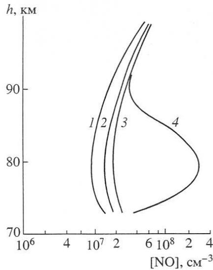
Fig. 2. The calculated [NO] height distribution for winter anomaly conditions (4), for medium (2), low (1) and high (3) solar activities.
