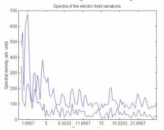
Figure 2. The spectral content of the components of electric field variations. The zero level for Y-component spectrum is brought up to 50 units. Clear spectral peak at 1.67 mHz is seen in the variations of Y-component.
