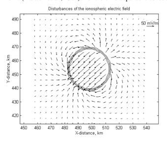
Figure 3. The ionospheric electric field disturbances in the vicinity of the heated area. The region of the enhanced conductivity is shown with triple line. The scaling vector of 50 mV/m is in the top right corner (after Pashin et al., 2000).
