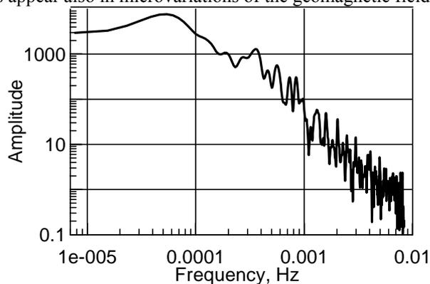
Fig. 5. The spectrum of power of a 6 hour data sequence of an amplitude of the geomagnetic field H-component at the Loparskaya observatory (16-22 UT, 24.09.2002)
