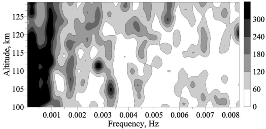
Fig. 3. The altitude behaviour of the spectrum of power of amplitude fluctuations for an hourly sequence of data (22:50 - 23:50 UT) in September 24, 2002.
