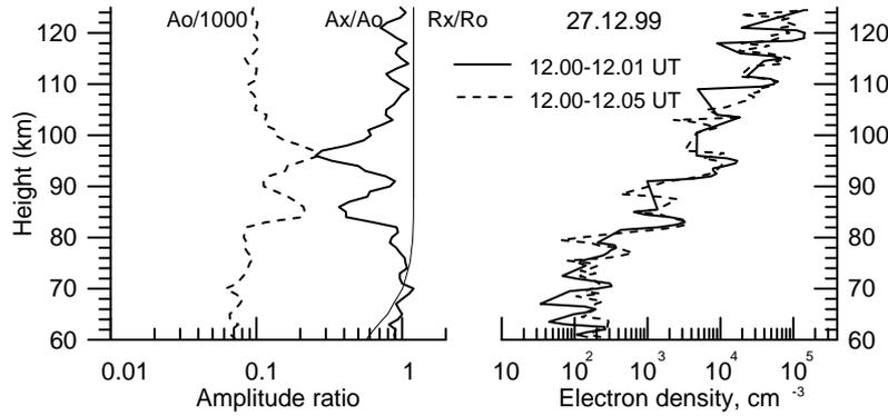
Fig.2. Profile of  $A_o/1000$ ,  $A_x/A_o$  and  $R_x/R_o$  for 2.7 MHz, and electron density  $N$  derived from these results.
