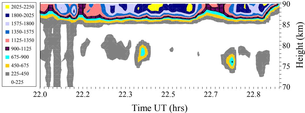
Fig.3. Time – altitude picture of the echo amplitude of O-mode 07.08.99.
