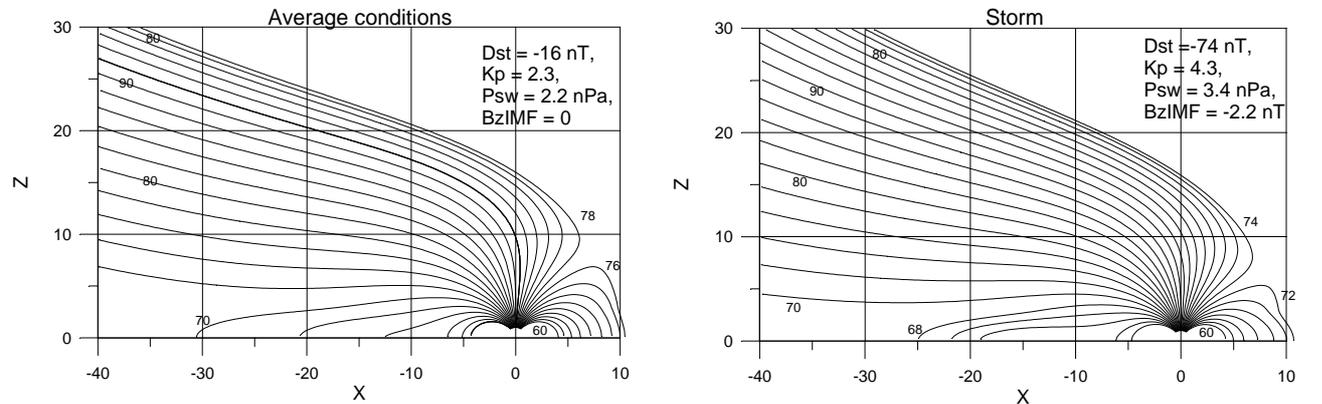
Fig. 2. The model magnetic field lines in the noon-midnight meridian plane for average (the left panel) and storm (the right panel) conditions.
